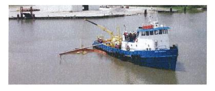
The VOSS (yellow) is being deployed and connected to an out-rigged arm. This is suitable for collection in both large pockets of oil and for recovery of streaming oil. The oil-to-skimmer encounter rate is limited by the length of the arm. Skimming pace is  $\leq 1$  knot.
