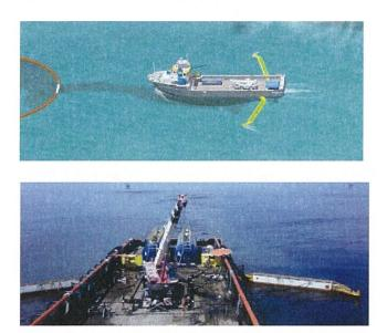
This is a depiction of the same operation as above but using KOSEQ Arms. In this configuration, the collecting boom speed dictates the operational pace at  $\geq 1$  knot to minimize entrainment of the oil.
