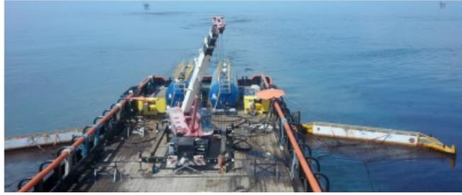
This is a depiction of the same operation as above but using KOSEQ Arms. In this configuration, the collecting boom speed dictates the operational pace at  $\geq 1$  knot to minimize entrainment of the oil.
