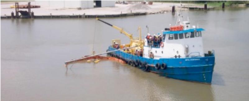
The VOSS (yellow) is being deployed and connected to an out-rigger arm. This is suitable for collection in both large pockets of oil and for recovery of streaming oil. The oil-to-skimmer encounter rate is limited by the length of the arm. Skimming pace is  $\leq 1$  knot.
